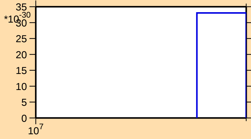
\sigma vs. E for ^{11}\text{Be}(n,n\alpha)
