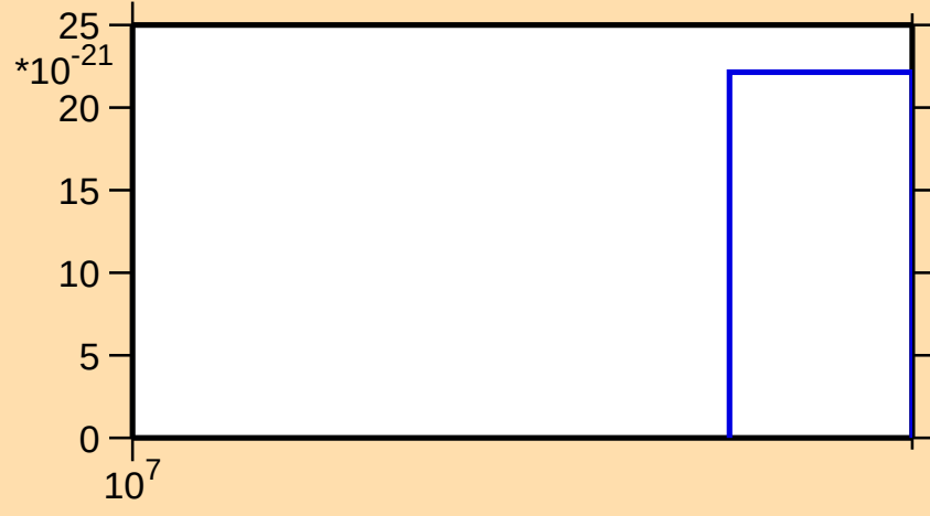
\sigma vs. E for ^{91}\text{Rh}(n,\text{nt})
