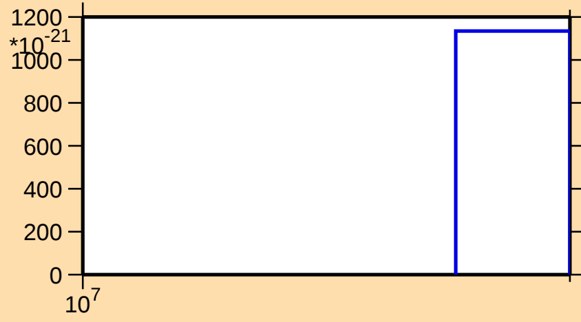
\sigma vs. E for ^{226}\text{Rn} (mt 42)
