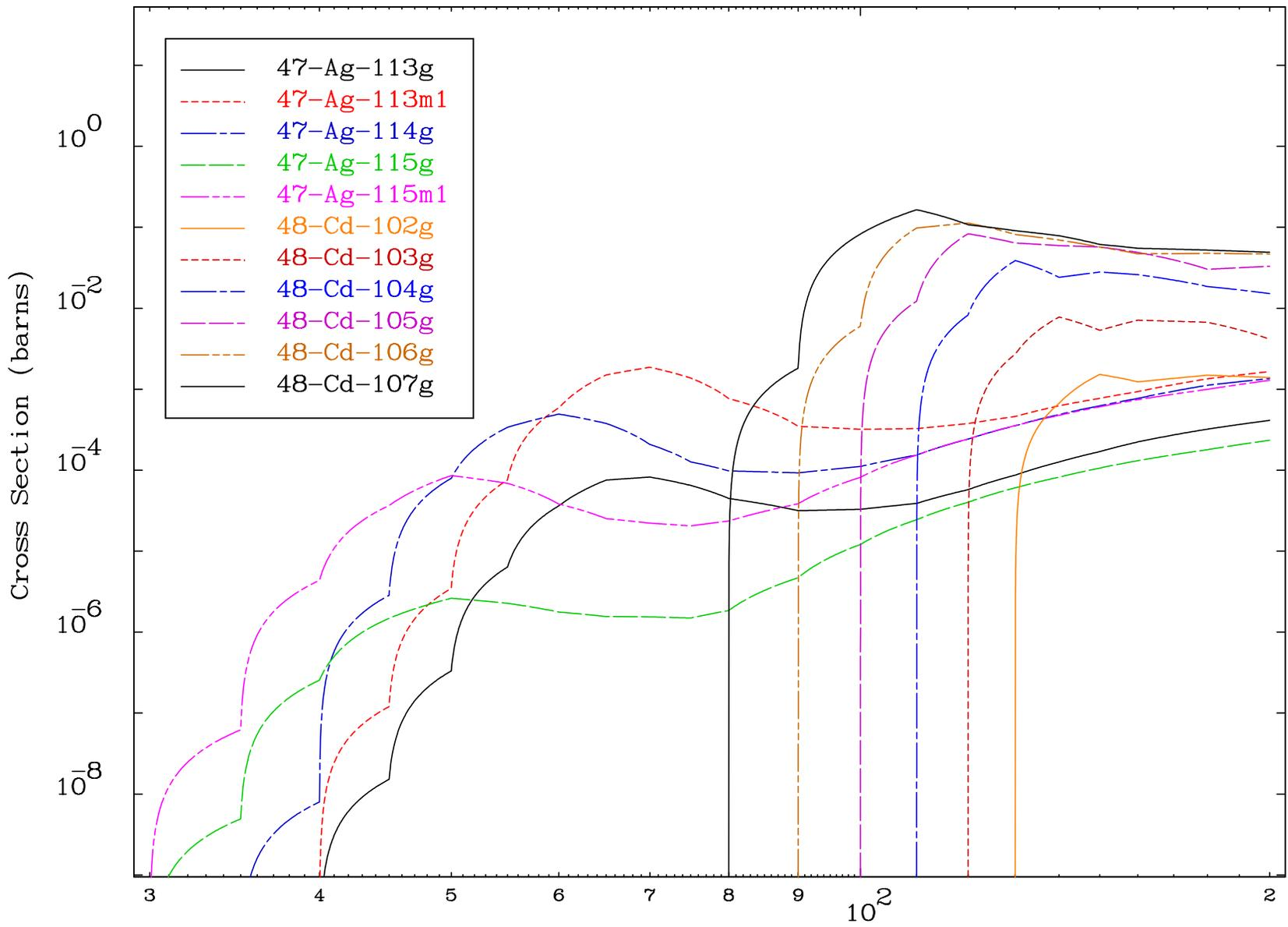
Radionuclide Production Cross Section
