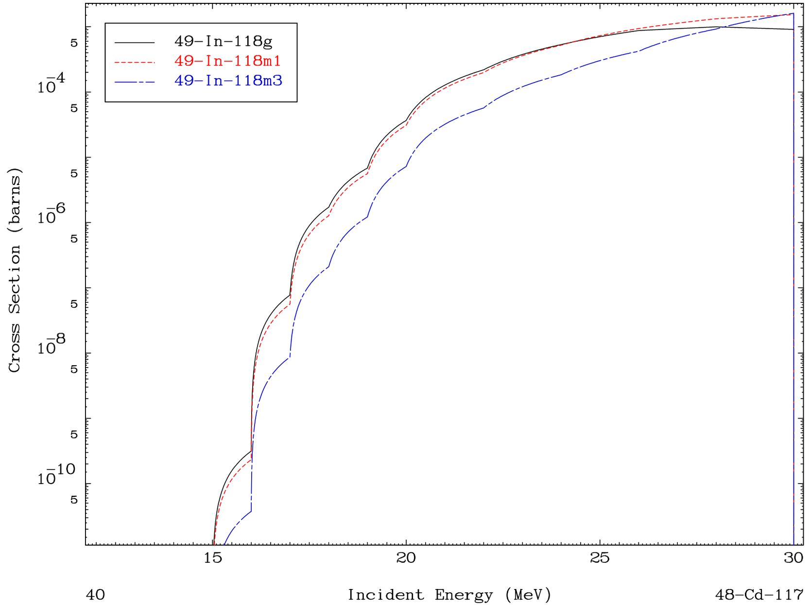
Radionuclide Production Cross Section
