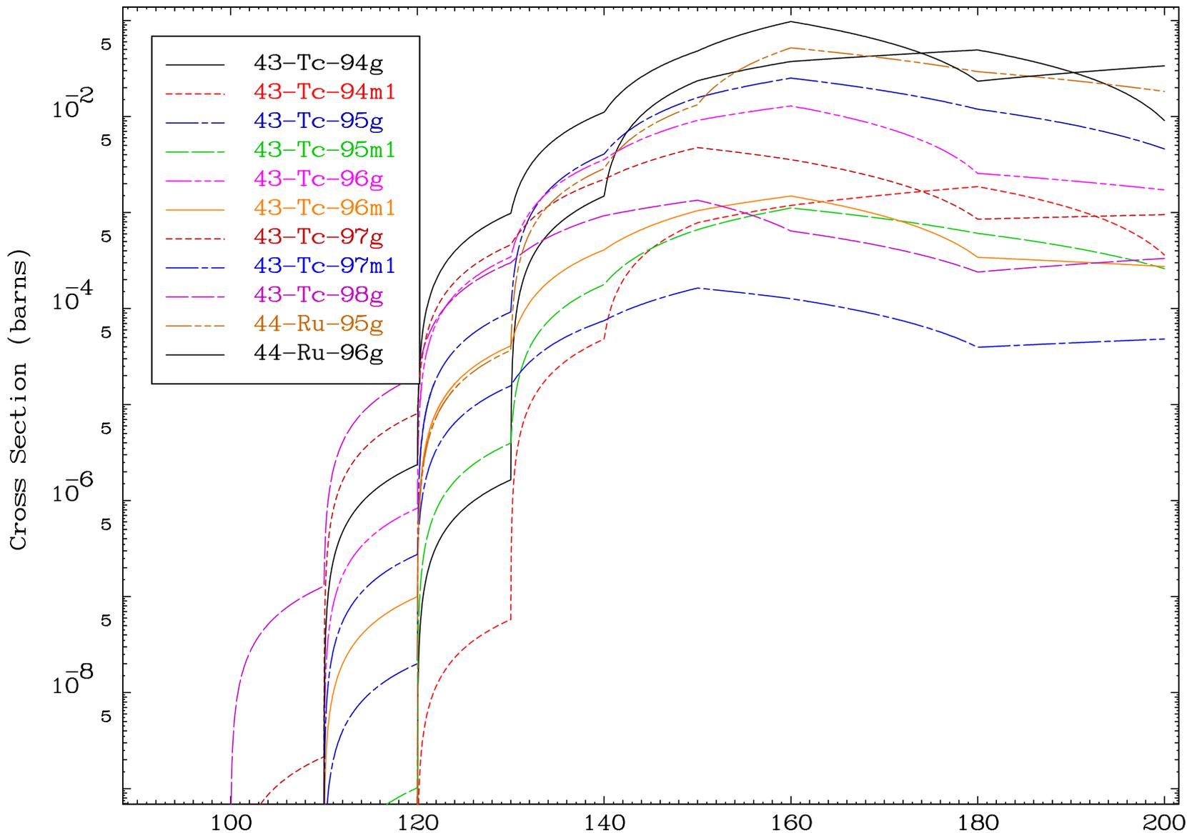
Radionuclide Production Cross Section
