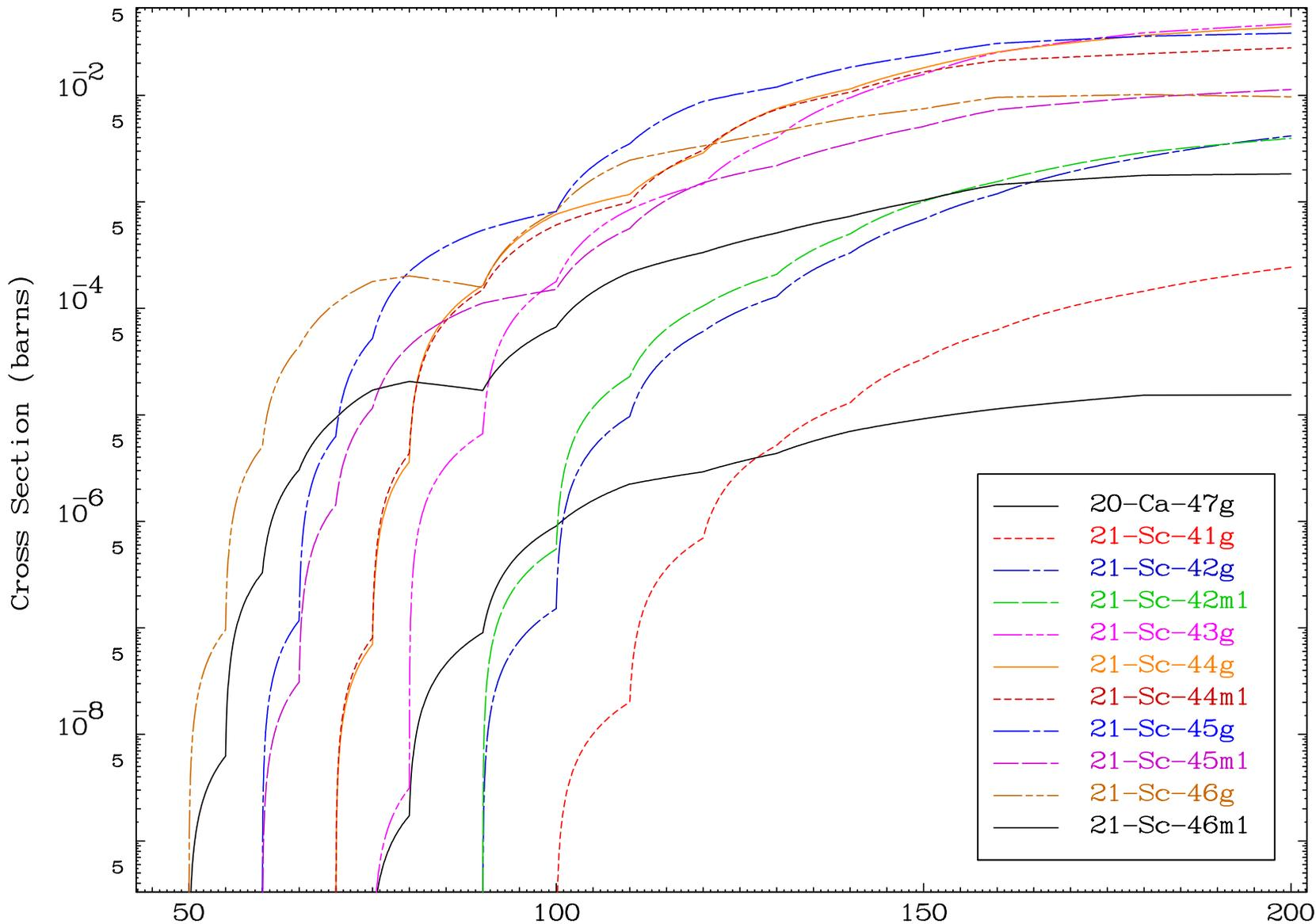
Radionuclide Production Cross Section
