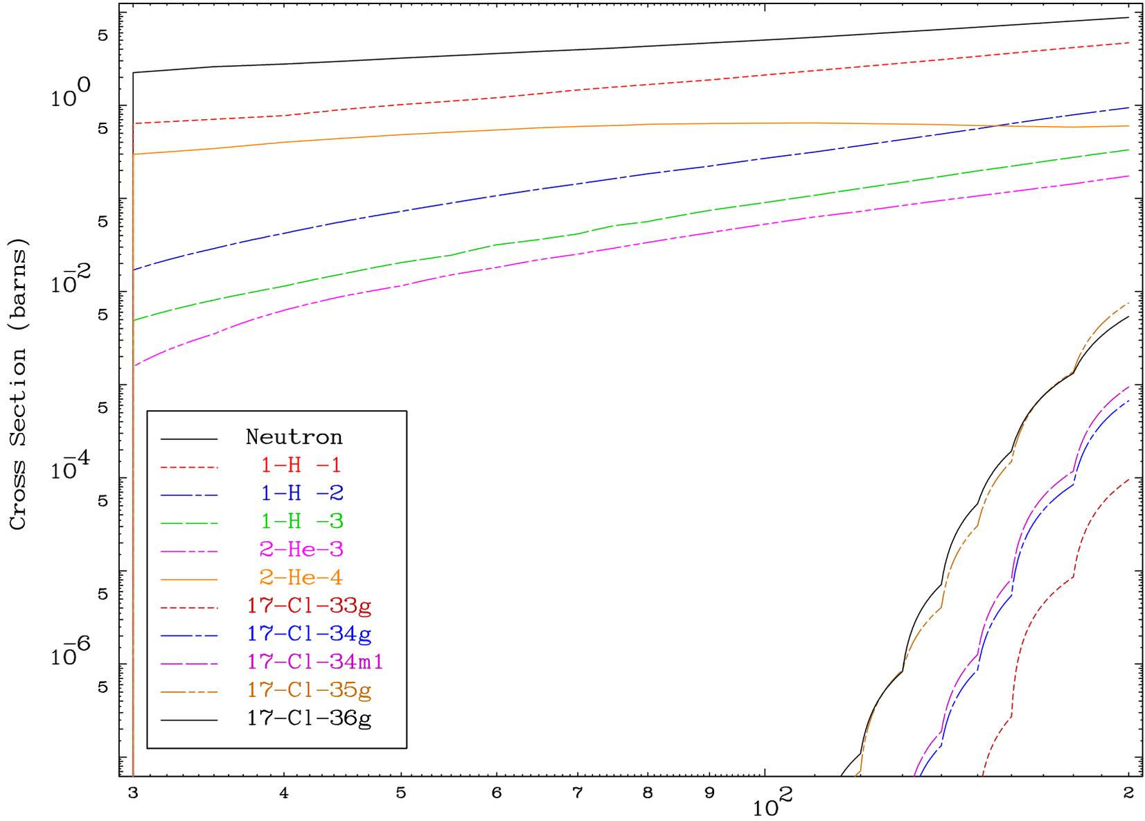
Radionuclide Production Cross Section
