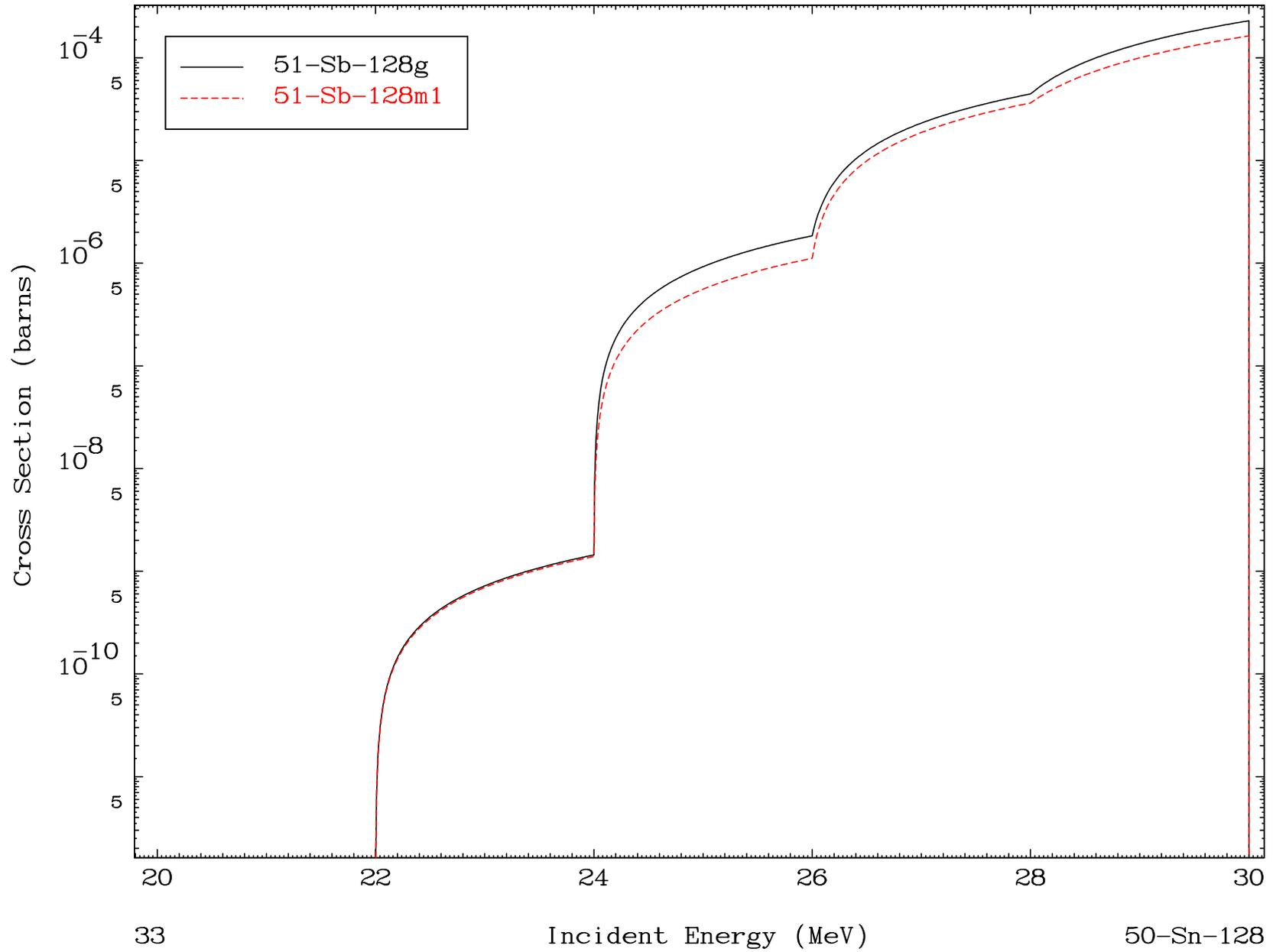
Radionuclide Production Cross Section
