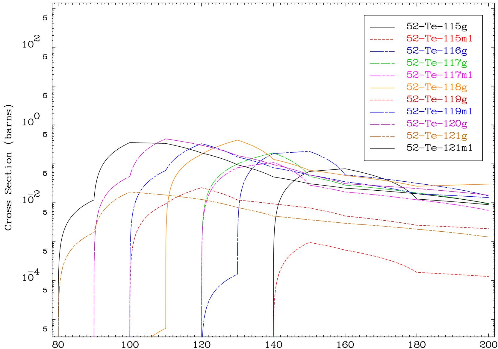
Radionuclide Production Cross Section
