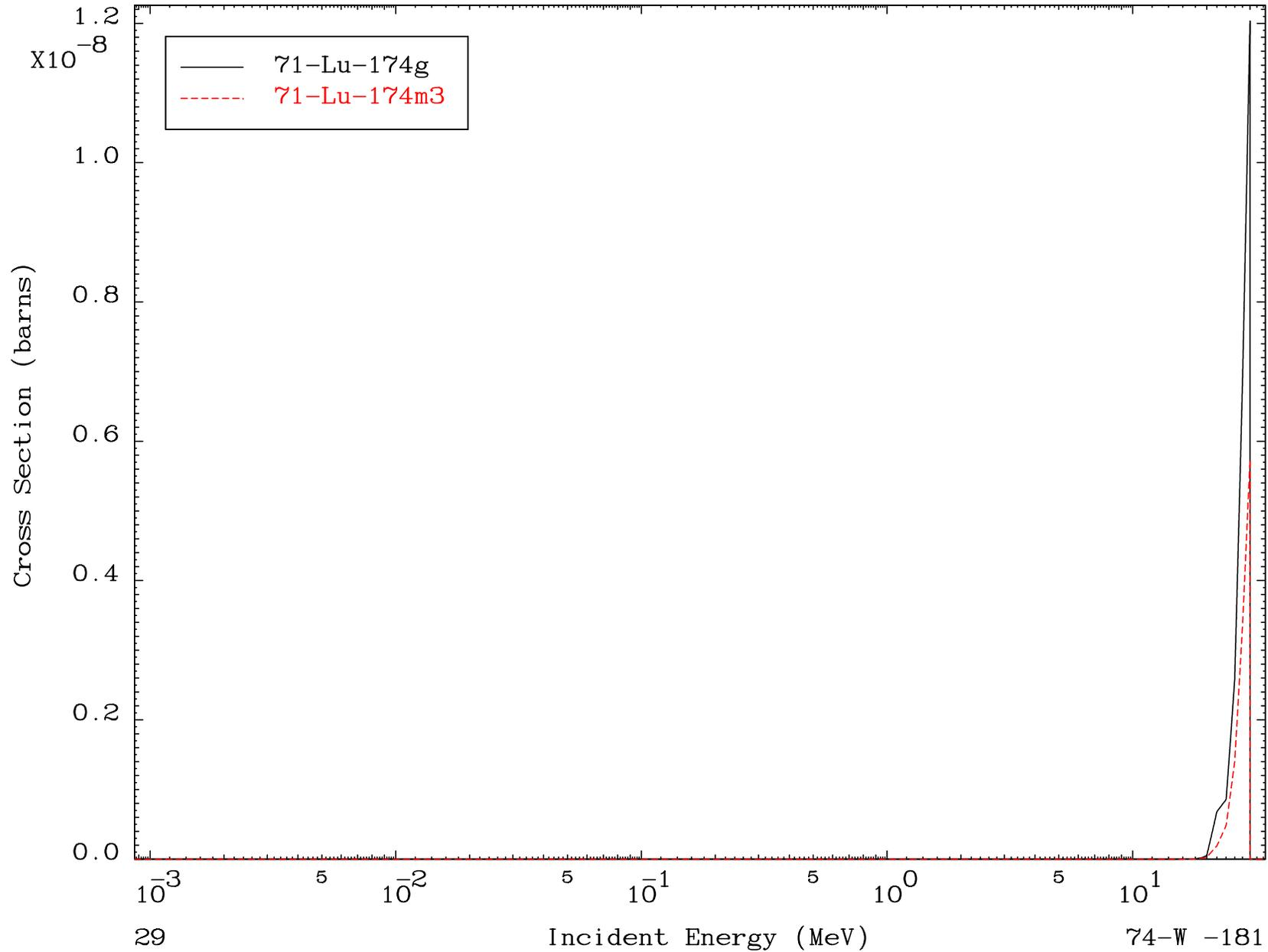
Radionuclide Production Cross Section
