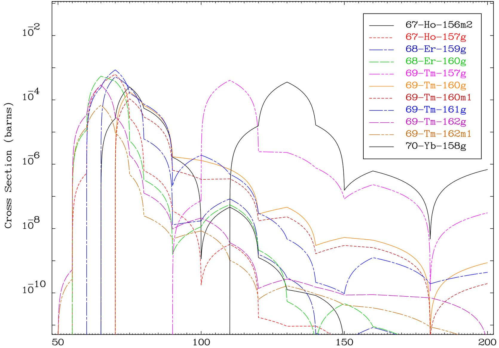
Radionuclide Production Cross Section
