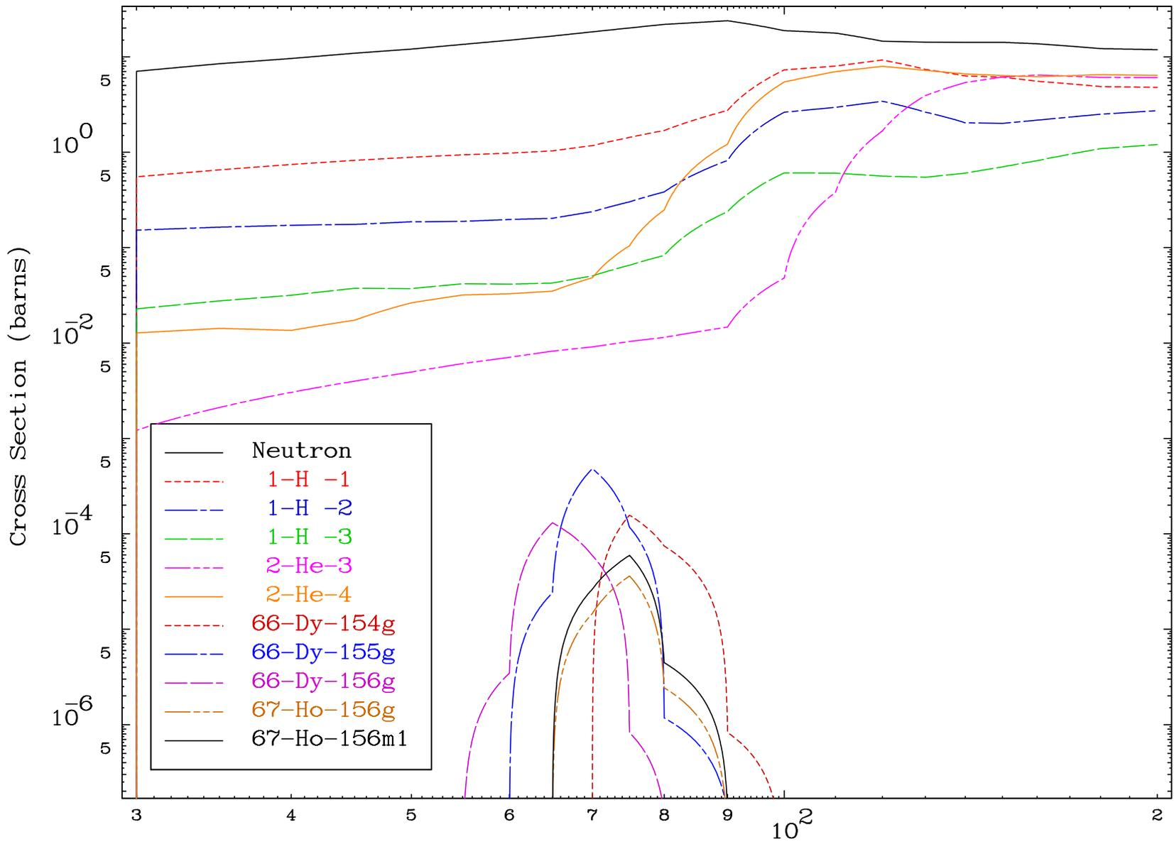
Radionuclide Production Cross Section
