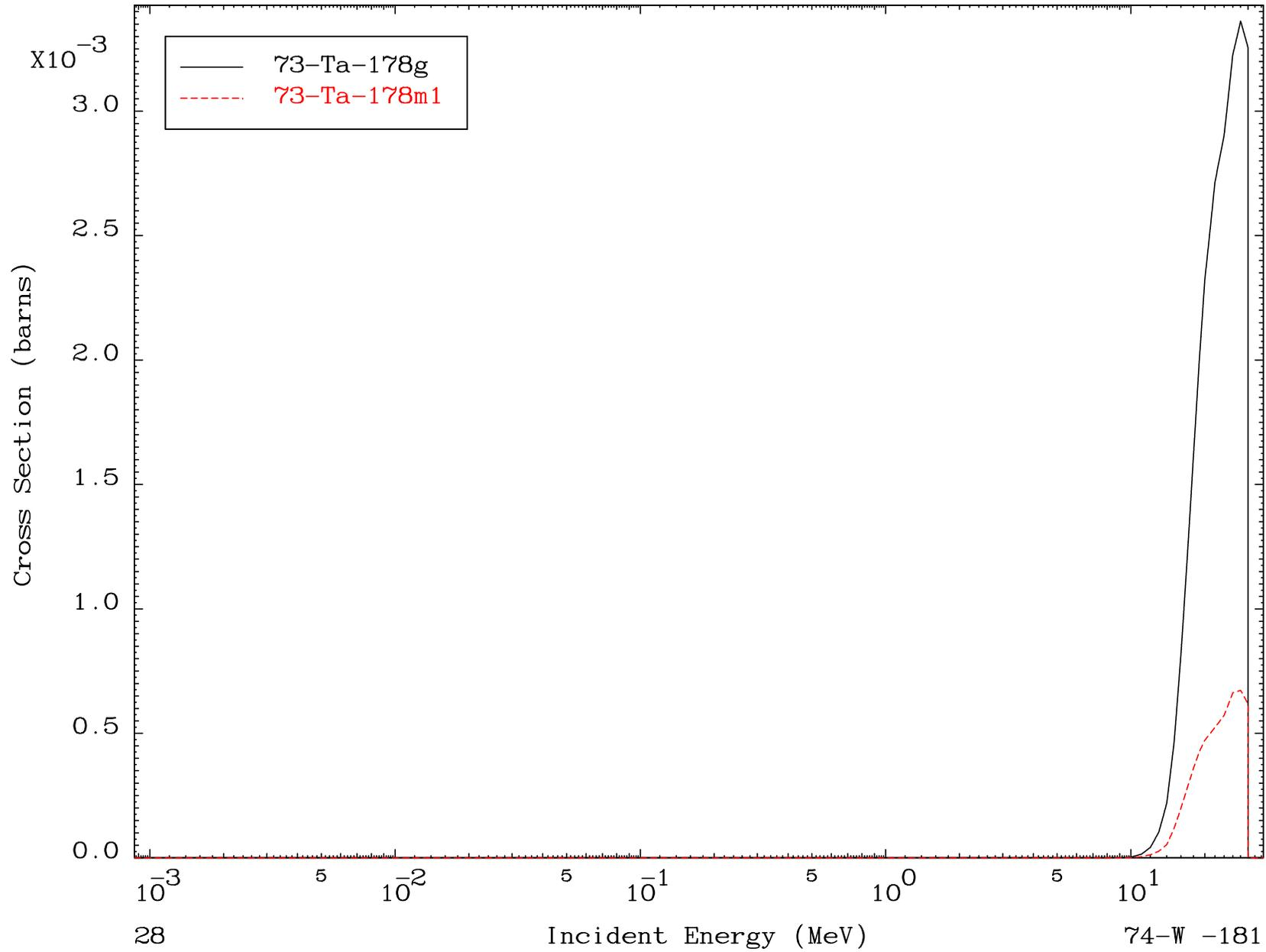
Radionuclide Production Cross Section
