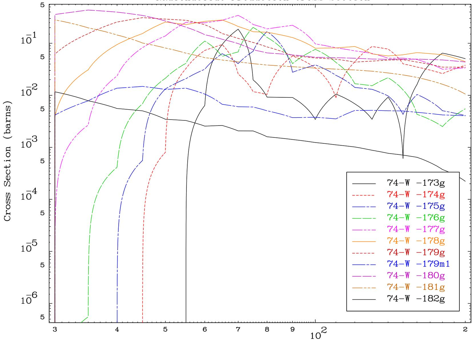
Radionuclide Production Cross Section
