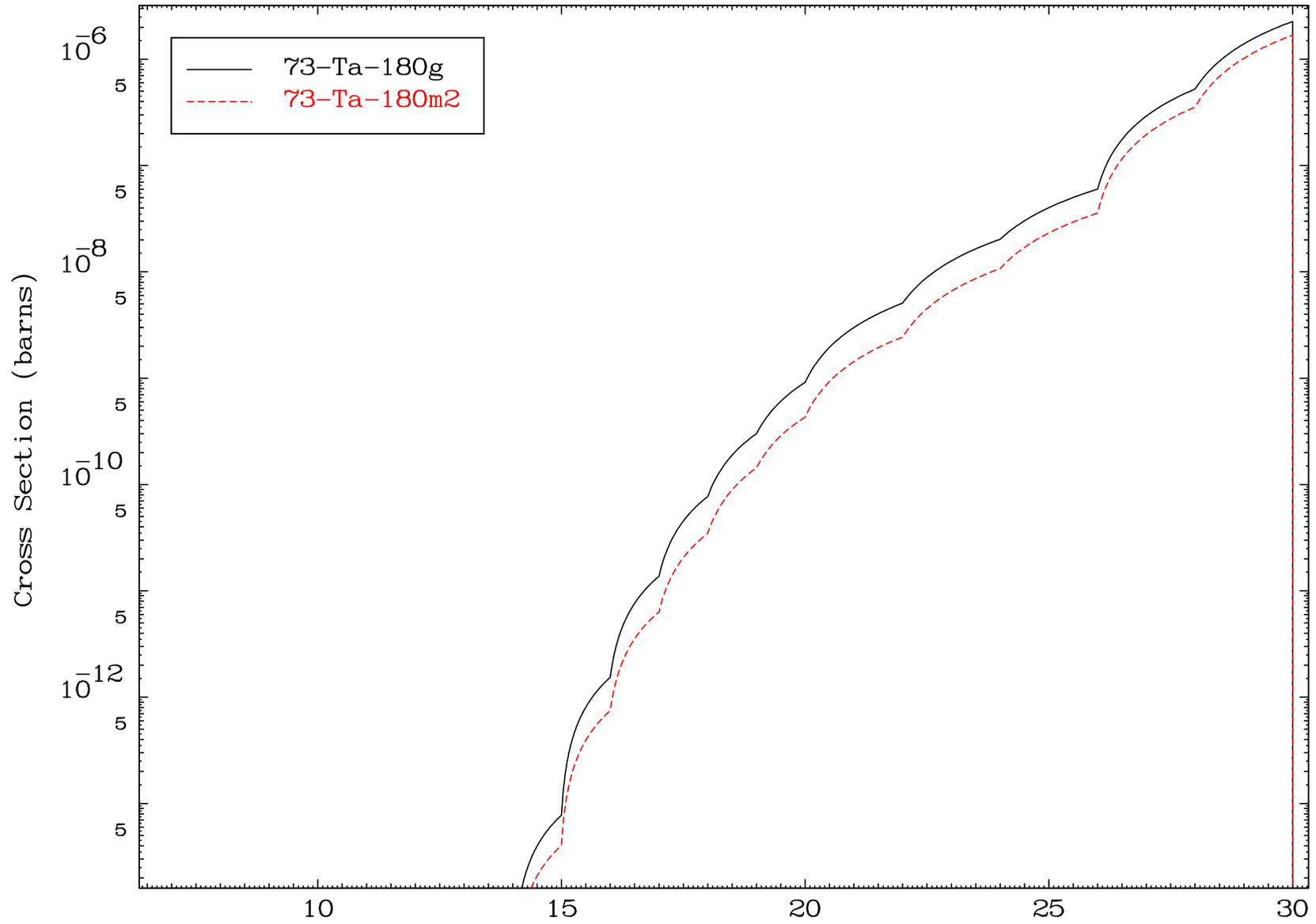
Radionuclide Production Cross Section
