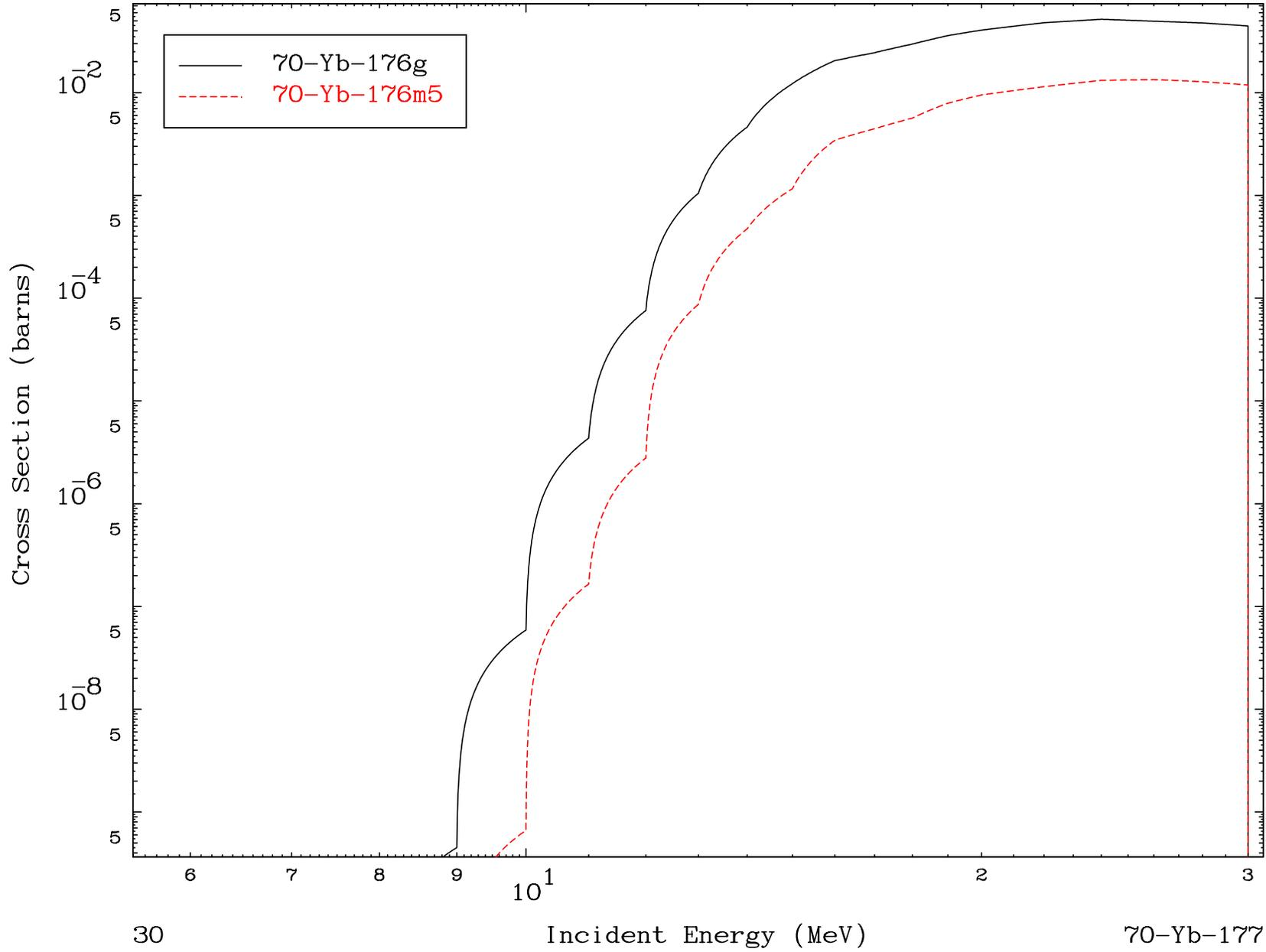
Radionuclide Production Cross Section
