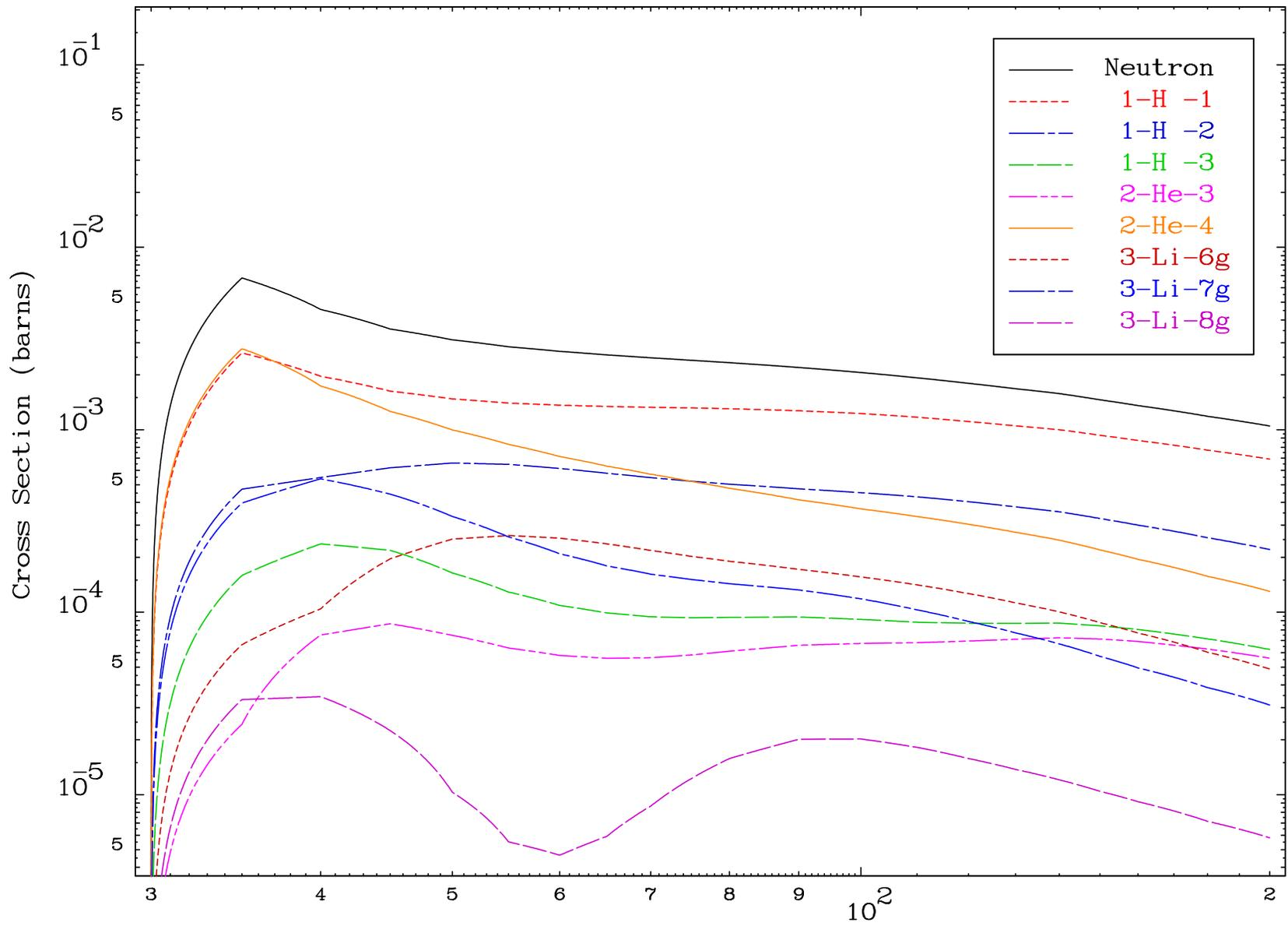
Radionuclide Production Cross Section
