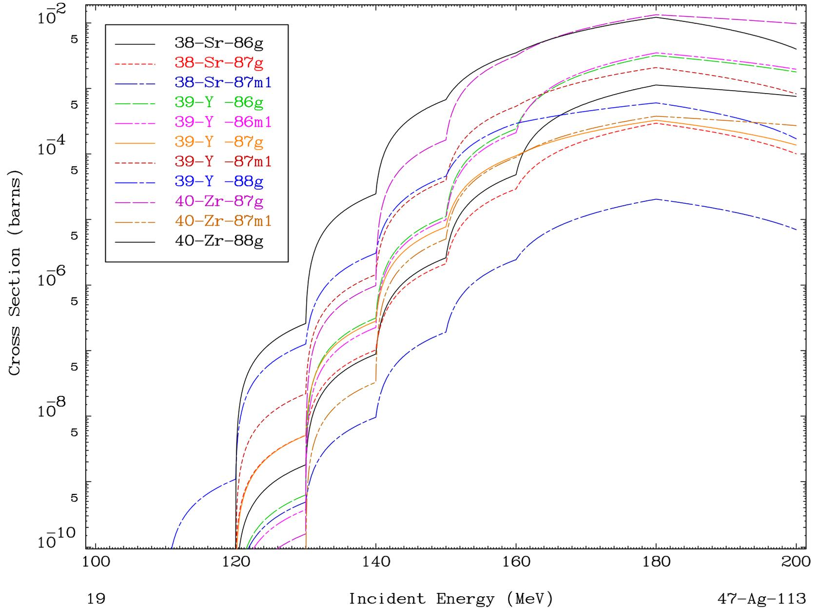
Radionuclide Production Cross Section
