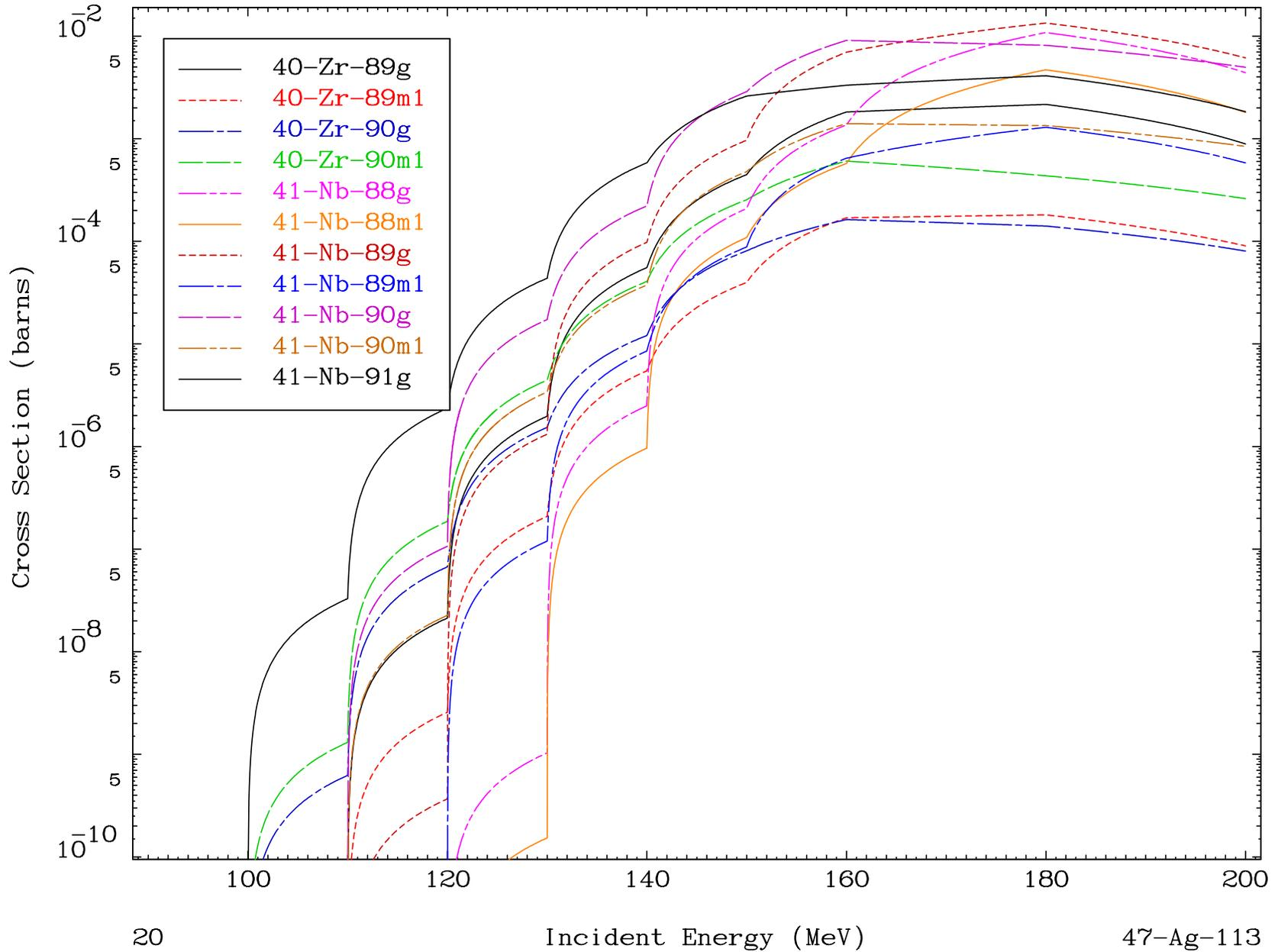
Radionuclide Production Cross Section
