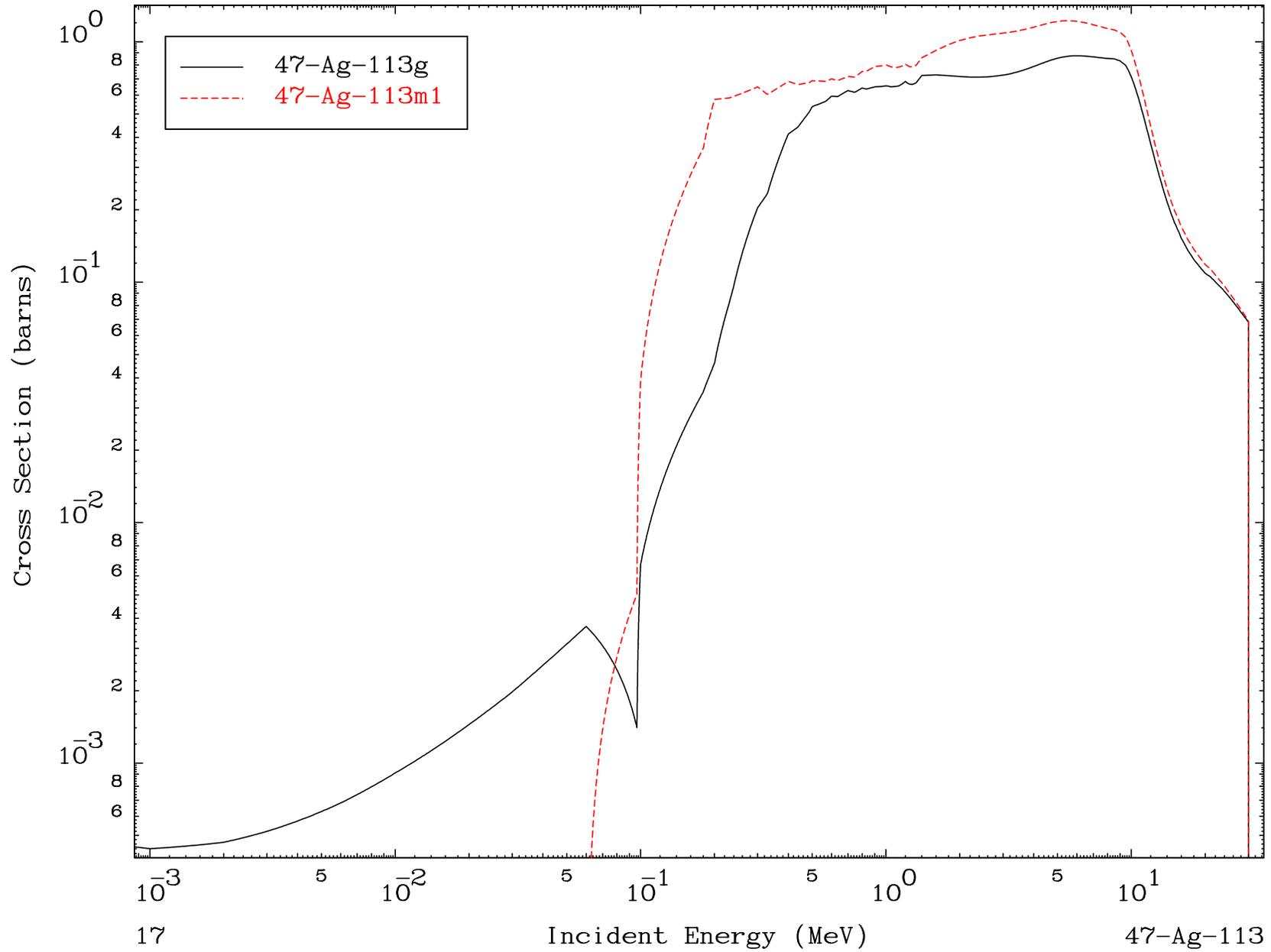
Radionuclide Production Cross Section
