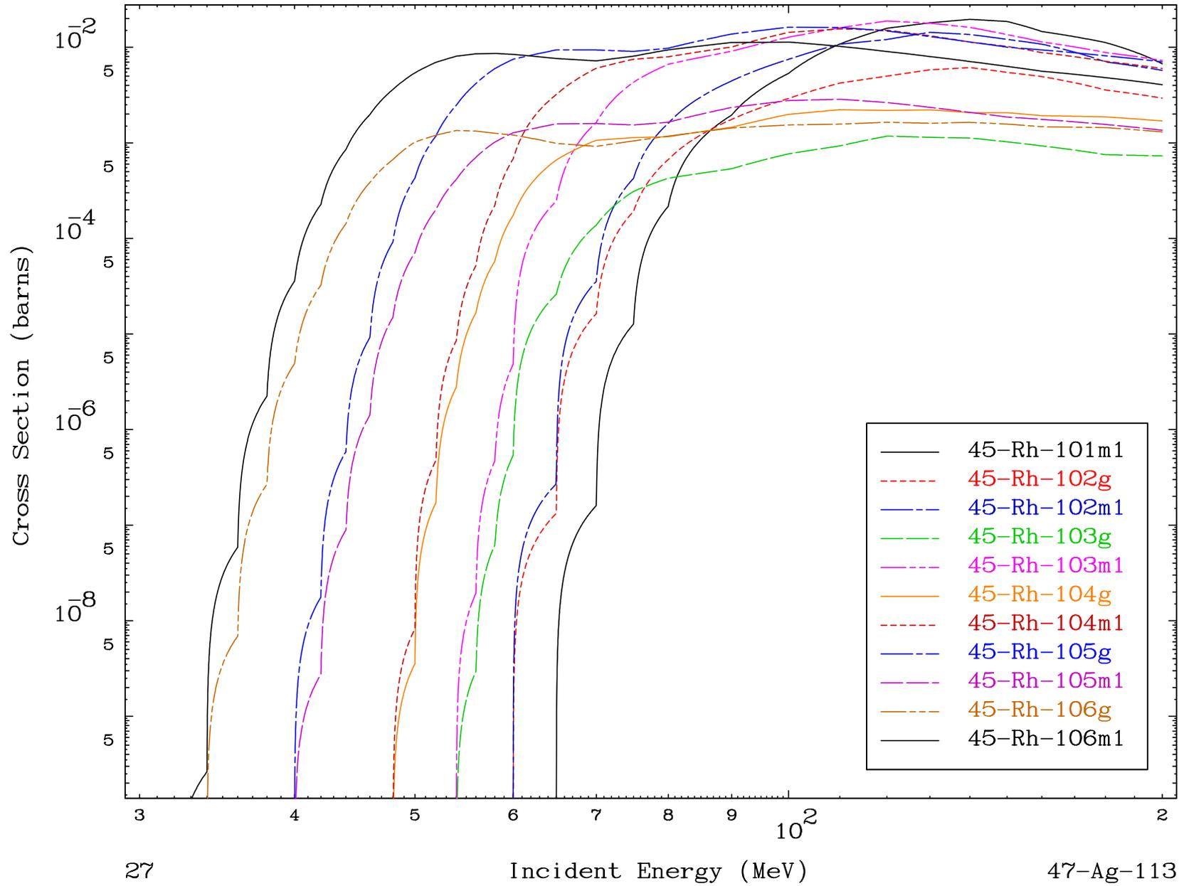
Radionuclide Production Cross Section
