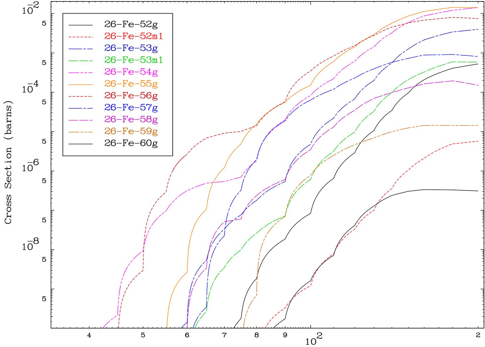
Radionuclide Production Cross Section
