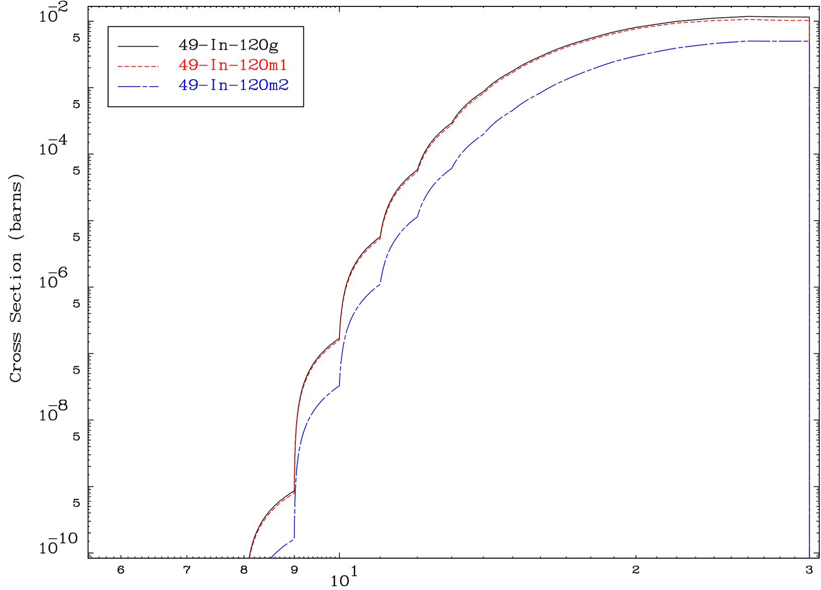
Radionuclide Production Cross Section
