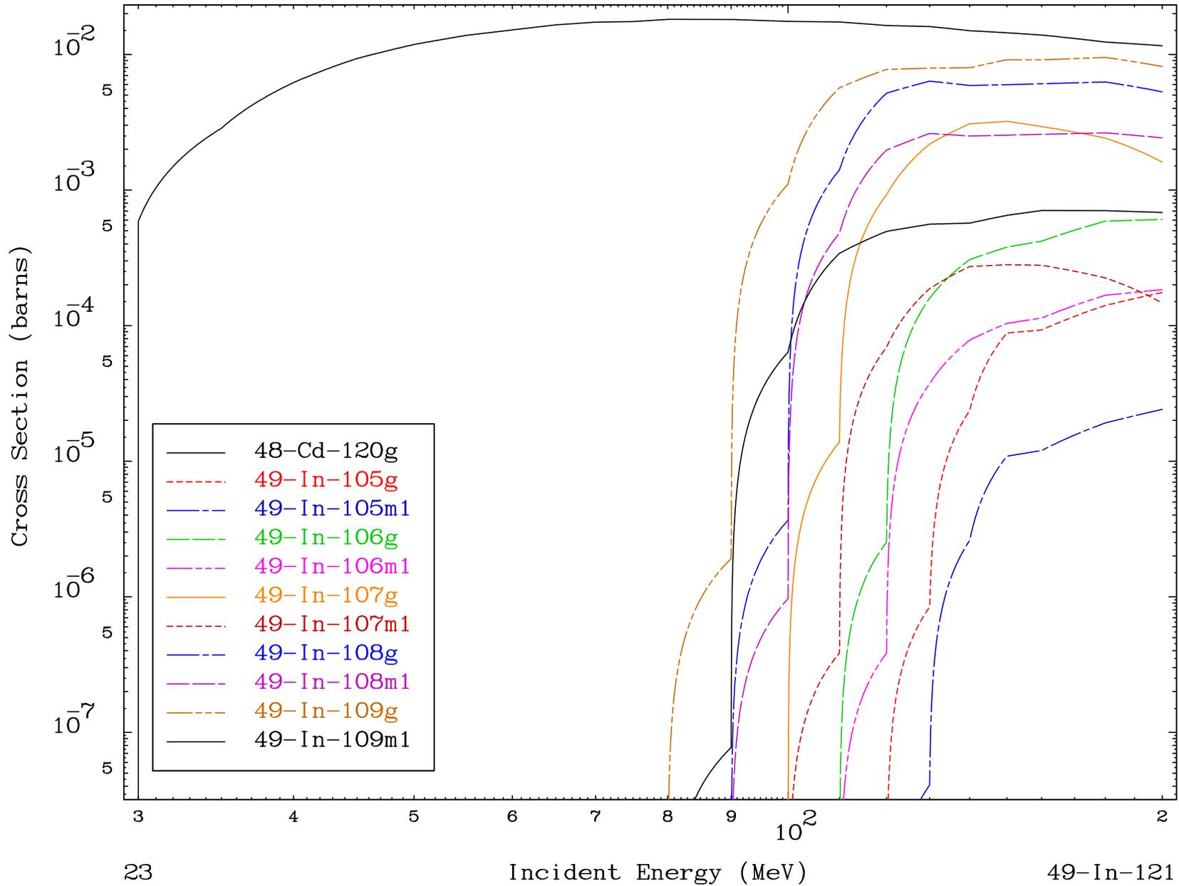
Radionuclide Production Cross Section
