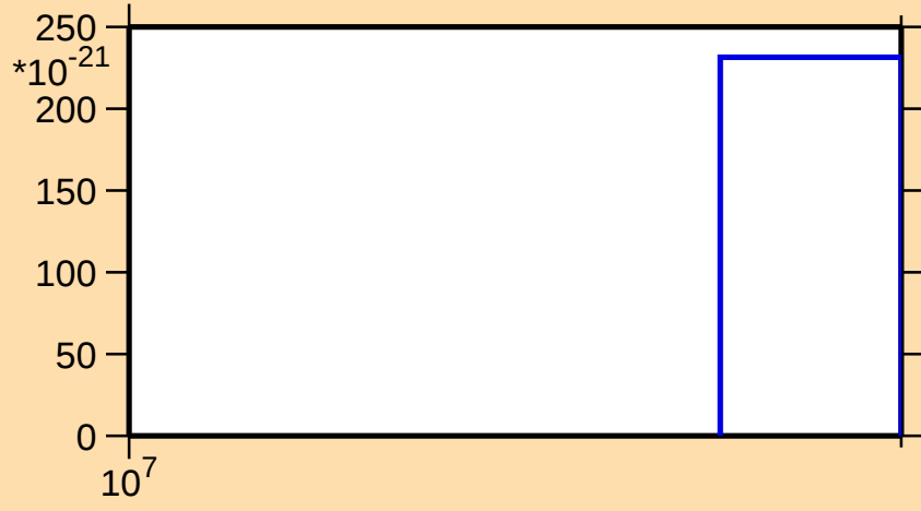
\sigma vs. E for ^{126}\text{Sb} (mt 11)
